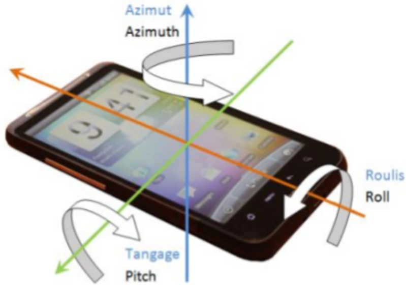
Figure 3: The angle definitions used by Android accelerometers.
